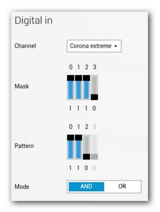
The sequence will be launched when a predefined state occurs on a digital input channel.
