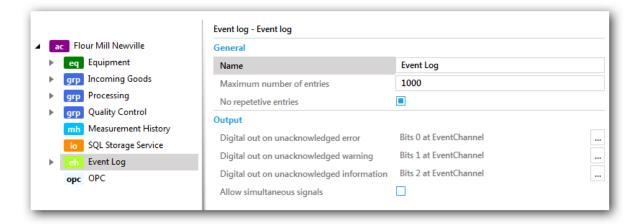
By activating the option "Allow simultaneous signals", the bit patterns of the different message types are set independently. By default, this option is deactivated, i.e. only the bit pattern of the severest message type is signaled.
