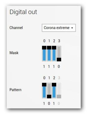
Assigns a predefined state to a digital output channel.
