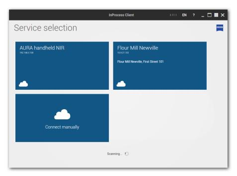
In case devices with an embedded controller, e.g. AURA handheld NIR, are connected to the computer or in case computers with a running InProcess-service are present somewhere in the network, entries for these network services will be shown. The selection of such a service establishes a network connection with the embedded controller or the remote computer. The user then arrives at the login screen, and the "InProcess Client" program behaves just like the standard "InProcess" program.
