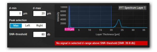
If it is not possible to catch the desired peak for various samples through the selection of  $\lambda$ -min and  $\lambda$ -max as well as d-min and d-max, the option Peak selection should be used. The options Left and Right enables the selection of the peak for the thinnest and for the thickest layer, respectively, in the range between d-min and d-max.
