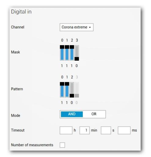
Stops the measurement when a defined state occurs on a digital input channel.
